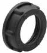
Used with locknut to protect conductors inside threaded rigid or IMC conduit entering a box. Rounded surface of bushing prevents damage to wire insulation.
