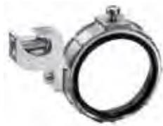
Used with locknut to terminate service conduit or fittings to cabinet. Tin Plated Aluminum alloy lug provided for bonding jumper to neutral busbar. Plastic liner prevents damage to wire insulation.
