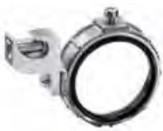
Used with locknut to terminate service conduit or fittings to cabinet. Tin Plated Aluminum alloy lug provided for bonding jumper to neutral busbar. Plastic liner prevents damage to wire insulation.
