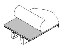
4. Place the brackets at the specified location and make sure the SS Butyl attaches well to the roofing surface. Set the bracket with 5 ea. (for Roof deck), of M6.0 $\times$ 60 mm stainless wood screws.
