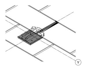
\* When there is a slit above the bracket, fill it is with SS Butyl to match its shape 3. If there is a shingle gap (tab shingles only) within 2 inches from the base, sealant or SS butyl shall be applied to the gap as it is shown.
