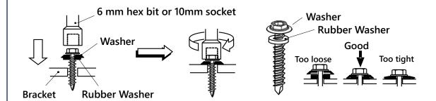
When tightening the screws please tighten all screws equally. Additionally, avoid using an impact driver as it can over torque the screws causing them to strip the threads.
