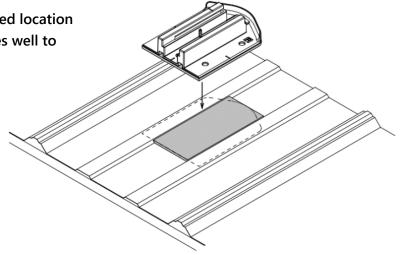
(4) Set the bracket with 5 ea. (For Roof Deck), of M6.0  $\times$  60 mm stainless wood screw using 6 mm hex bit. After completing the process, make sure the brackets are securely fixed.
