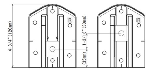
1. Locate and place SSB1 base on the cross section of chalk line.
