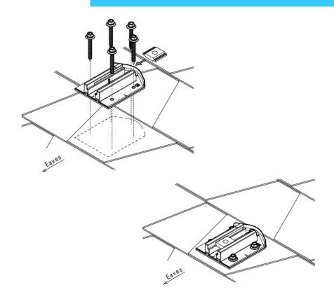
Place the brackets at the specified position and make sure the SS Butyl makes good contact with the roofing surface.
