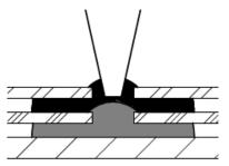
(5) Set the bracket with 5 ea. (For Roof Deck), of M6.0 x 60 mm stainless wood screw using 6 mm hex bit or 10mm socket.
