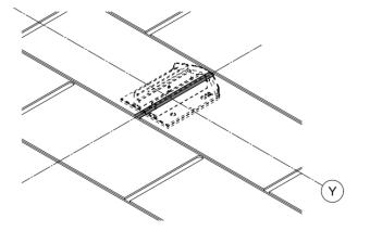
\* (for tab shingles only) When there is a slit at the installation spot, fill in with the additional SS butyl tape. The slit must be filled with SS Butyl.
