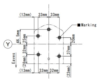
3. Do not drive the M6  $\times$  60 screw on the butyl spacer location. Apply the butyl spacer if the base is installed in the shaded area.
