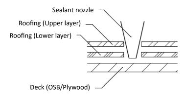
(3) Fill sealant layer by layer. Hold the nozzle in place to ensure lowest layer is filled with sealant displacing all air around the desired attachment point.
