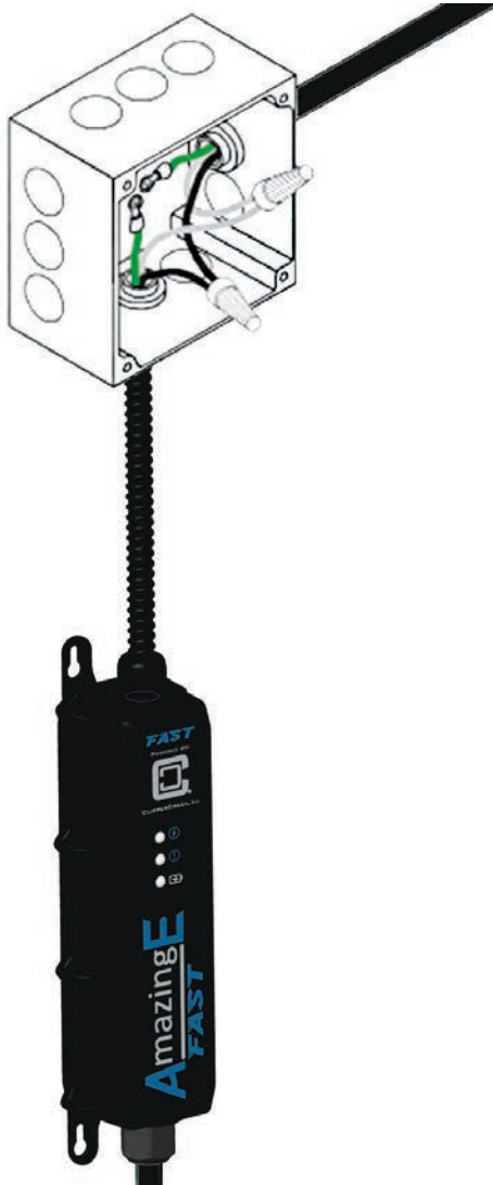
Figure 7: Wiring the EVSE in a junction box
