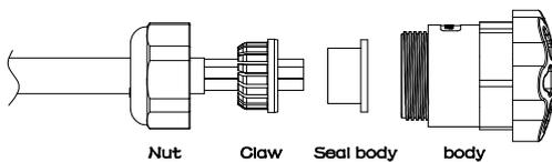
c. Insert five wires into the core wires hole of the body.
