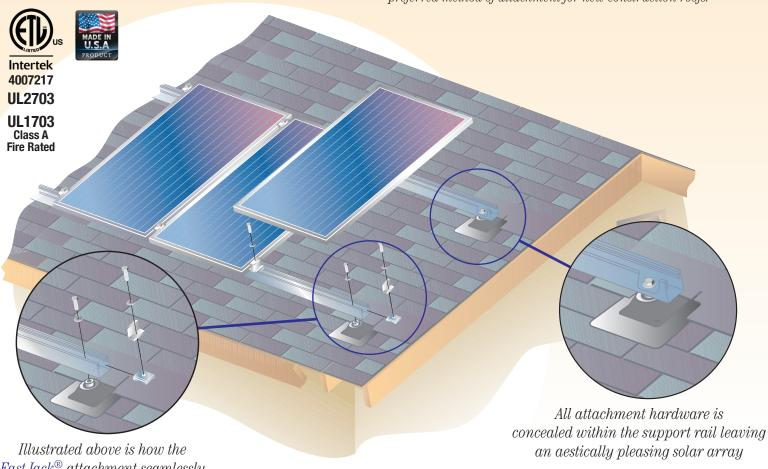
Illustrated above is how the FastJack® attachment seamlessly integrates with the RoofTrac® mounting system.
