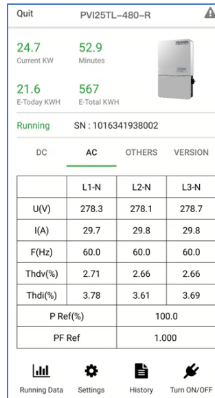
Figure 4-5 Normal Operation Status
