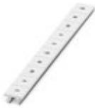
Marker for terminal blocks, Strip, white, labeled, can be labeled with: CMS-P1-PLOTTER, horizontal: U, V, W, N, GND, U, V, W, N, GND, mounting type: snap into tall marker groove, for terminal block width: 10.2 mm, lettering field size: 10.15 x 10.5 mm, Number of individual labels: 10
