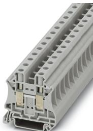
Feed-through terminal block, nom. voltage: 1000 V, nominal current: 57 A, connection method: Screw connection, Rated cross section: 10 mm<sup>2</sup>, cross section: 0.5 mm<sup>2</sup> - 16 mm<sup>2</sup>, mounting type: NS 35/7,5, NS 35/15, color: gray
