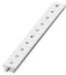
Marker for terminal blocks, Strip, white, labeled, can be labeled with: CMS-P1-PLOTTER, horizontal: L1, L2, L3, N, PE, L1, L2, L3, N, PE, mounting type: snap into tall marker groove, for terminal block width: 10.2 mm, lettering field size: 10.15 x 10.5 mm, Number of individual labels: 10
