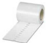
Marker for terminal blocks, Roll, white, unlabeled, can be labeled with: THERMOMARK ROLL 2.0, THERMOMARK ROLL, THERMOMARK ROLL X1, THERMOMARK ROLLMASTER 300/600, THERMOMARK X1.2, THERMOMARK S1.1, perforated, mounting type: snap in, snap into flat marker groove, for terminal block width: 10.2 mm, lettering field size: 6.35 x 10.15 mm, Number of individual labels: 10000
