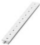
Zack marker strip, Strip, white, labeled, can be labeled with: CMS-P1-PLOTTER, Printed vertically: consecutive numbers 1 ... 10, 11 ... 20, etc. up to 91 ... 100, mounting type: snap into tall marker groove, for terminal block width: 10.2 mm, lettering field size: 10.15 x 10.5 mm, Number of individual labels: 10
